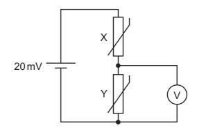
The cell has electromotive force (e.m.f.) 20 mV and negligible internal resistance.
