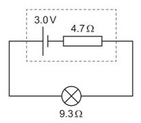
What is the power dissipated by the internal resistance of the cell?
